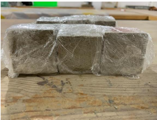
Figure 9: Sealing of the reference and alkali-activated slag mortar specimens in plastic wrapping for 27 days following thermal curing.
