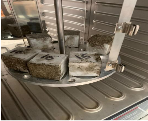
Figure 8: Thermal curing of the reference and alkali-activated slag mortar specimens in an incubator at 65 °C for 24 hours.
