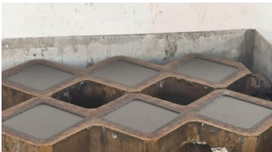
Figure 5: Casting of several alkali-activated slag mortar specimens.
