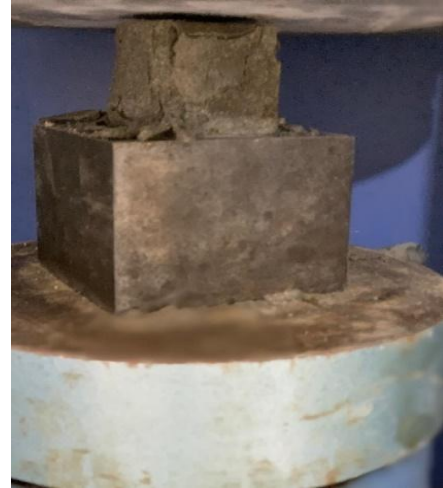
Figure 10: Compressive strength testing of a specimen at 28 days.
