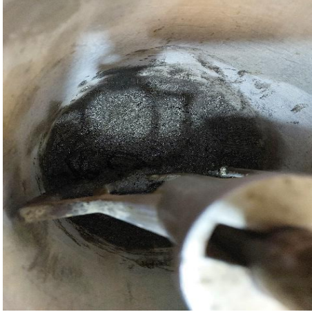
Figure 4: Mixing of an alkali-activated slag mortar specimen.
