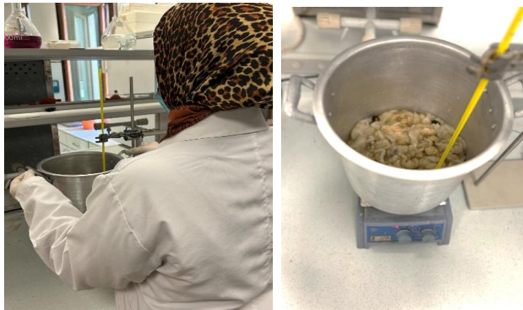
Figure 2. Preparation of wool treatment to extract lanoline.
