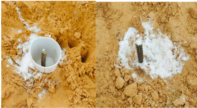
Fig. 7. Electrode with Sodium Chloride
