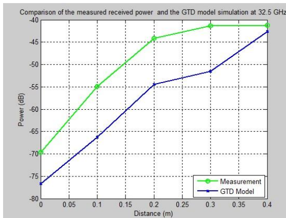
Fig.4. Modeled vs. Measured Received Power (Human Blockage Scenario).
