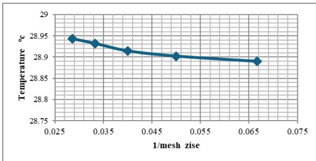
Fig. 4. convergence study of maximum temperature
