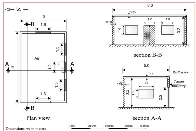
Fig 2: Room floor plan view & cross sections
