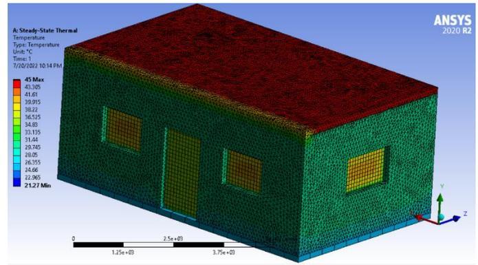
Fig. 5. Temperature distribution on the room envelop.
